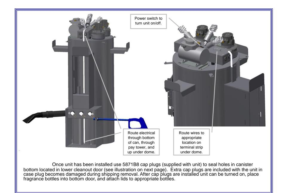
To attach hose, thread into metal hole counter clockwise.
