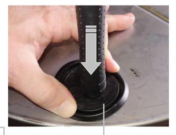
To insert 5871B8 cap plugs into bottom holes, pinch cap plug into place using index finger and thumb. With edges of plug resting against edges of hole, firmly push down on plug with end of hammer or other blunt object until plug snaps into place.
